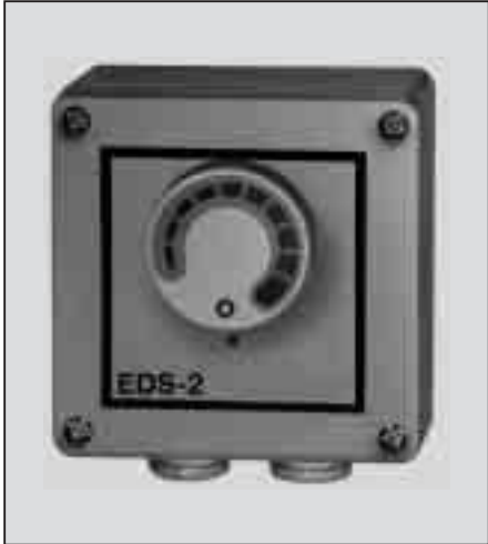
Electronic speed controller EDS 2 / EDS 2-Z for single-phase a.c. motors without thermal overload contacts and current ratings below 2 A. In its EDS 2 configuration this controller permits an infinitely variable manual speed adjustment; its EDS 2-Z counterpart allows any two fan speeds to be selected via a contacting unit. Suitable for DRH-Minivent and DRV-Minivent series fans. Available for concealed (UP) and apparent mounting (AP) (photo shows the AP type). Both versions conform to protection class IP 44 and are waterproof (WD).
