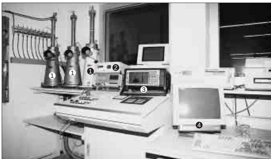
View of the measuring centre of our test station. The requisite array of high-precision instruments includes a Betz pressure gauge (1), a calibrating unit for the pressure
