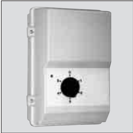
Speed controller R-ET Transformer-type speed controller for single-phase a.c. motors with external thermal overload contacts. May be used for manual speed-control in 5 stages with full motor protection. Connection of contacting unit and actuating motor is possible.
