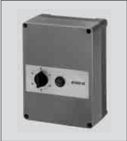
RTRD series speed controller Fans marked with an asterisk (*) in the specification tables are equipped with variable-speed motors. They can be speed-controlled in 5 stages via this controller (with full motor protection based on built-in thermal overload contacts). The fan speed can thus be reduced to about 50% of the nominal rpm value.
