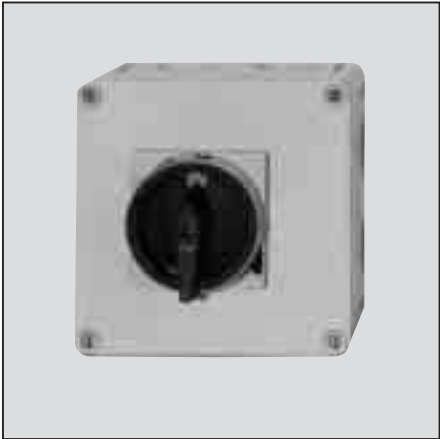
Local isolator Externally mounted and freely accessible, these switches are also equipped for special circuit configurations (e.g., three-lock interlocking, connection to a centralized control system, etc.). They can thus be used as emergency stop devices and are fully in compliance with VDE 0113 - IEC 204 and VGB 4 (standard except on BVD, DRV-F-K and hazardous duty fans).
