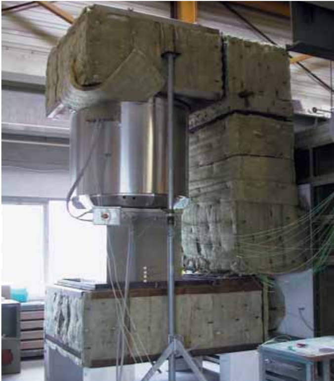
Complete test rig for roof-mounted smoke exhaust fans. Fumes are extracted from a furnace and returned to it via a duct connected to the fan outlet.
