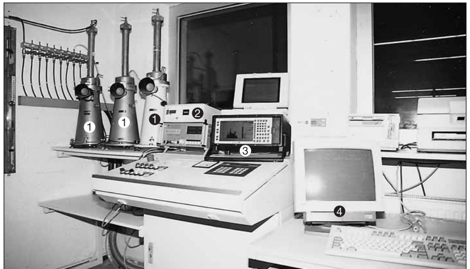
View of the measuring center of our test station. An array of high-precision instruments are needed for the measurements, e.g., a Betz pressure gauge ①, a calibration
