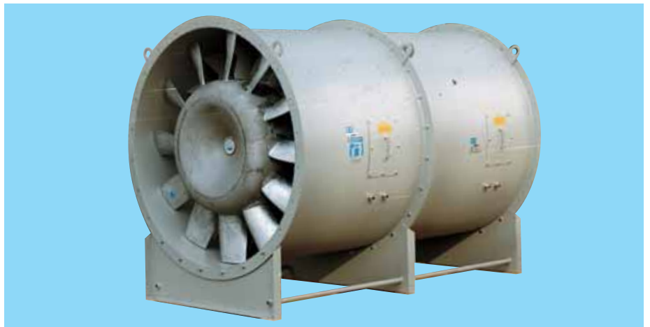
Two-stage axial flow fans, e.g., for car park ventilation or operation against high pressures, are a recent addition to our product range. These units are also available for 200° C / 300° C or 400° C – 120 min. operation (tested to EN 12101 – T3 standard specifications).
